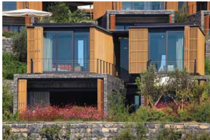
Thermowood-Claddings are long-lasting and stable, convenient for horizontal and vertical applications with its size and its various form. Thus, while supporting the design and aesthetic appearance of your buildings, it also provides a high resistance to extreme weather conditions.
